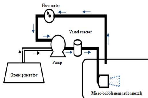
Figure 1. Schematic diagram of the Micro-bubbles Ozone system
