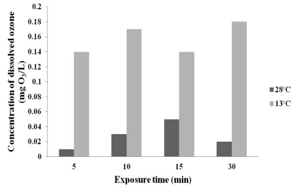
Figure 2. Concentrations of dissolved ozone in water was measured by Indigo colorimetric method at 28 and 13°C
